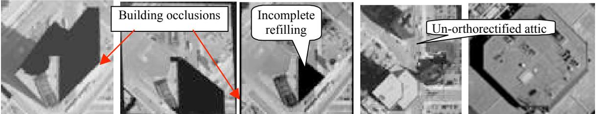
Fig. 4. Building occlusion in the master image (a) and in the slave image (b), and (c) result by refilling, (d) image position, and un-orthorectified image (d)
